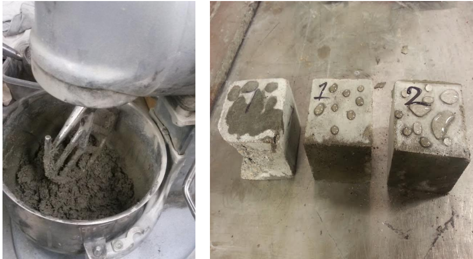
Figure 14. Left: Mixing sand, cement, and water Right: Water on control and PTFE-treated mortar samples.
